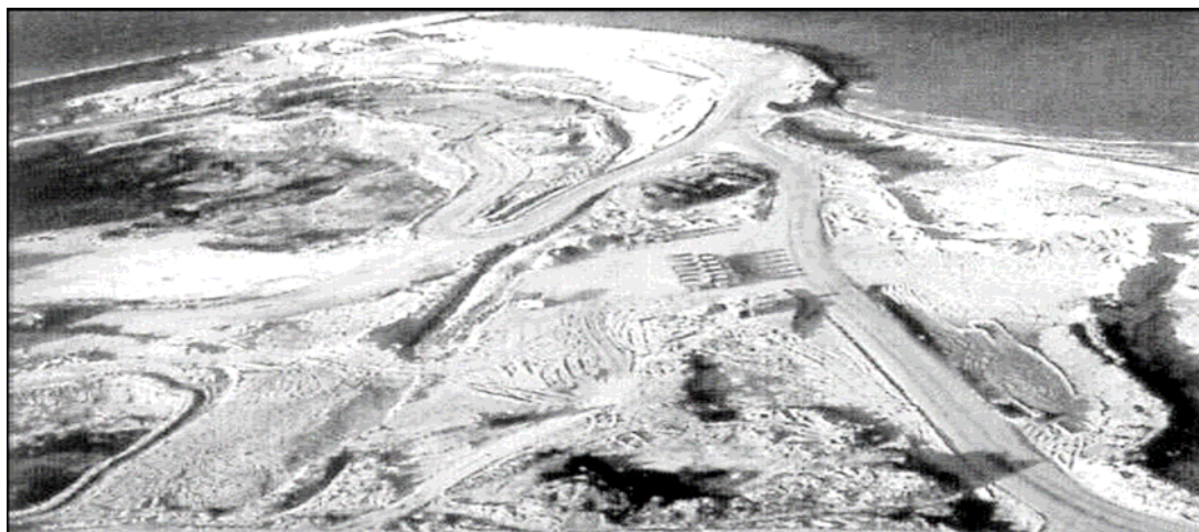
Figure 6. Coastline deformation due to mining operations on the Black Sea coast of Istanbul. (Courtesy of Istanbul Sand Miners Association, 1999)
