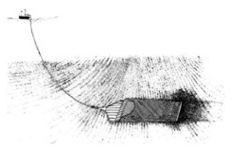
Figure 7. Action of a scallop and mussel dredge as it is dragged over a soft bottom seabed (DeAlteris et al., 1999).
